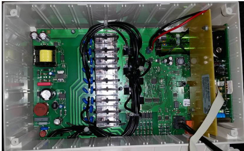
Fig. 1: proControl® 2 housing with GSM modem board on the right
