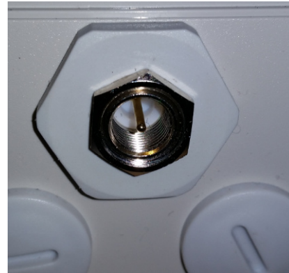
Fig. 4: FME-connector in cable gland
